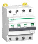
Residual current breaker with overcurrent protection (RCBO), Acti9 iC60, 4P, 32A, B curve, 6000A/6kA, A-SI type, 30mA
