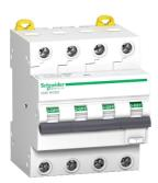
Residual current breaker with overcurrent protection (RCBO), Acti9 iC60, 4P, 25A, B curve, 6000A/6kA, A type, 30mA
