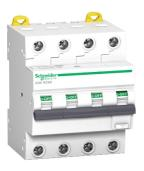
Residual current breaker with overcurrent protection (RCBO), Acti9 iC60, 4P, 16A, B curve, 6000A/6kA, A type, 30mA
