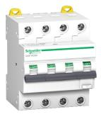
Residual current breaker with overcurrent protection (RCBO), Acti9 iC60, 4P, 32A, C curve, 6000A/6kA, AC type, 300mA
