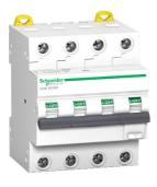
Residual current breaker with overcurrent protection (RCBO), Acti9 iC60, 4P, 20A, C curve, 6000A/6kA, A type, 300mA
