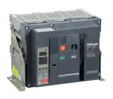
Circuit breaker frame, MasterPact NW32H2, 3200A, 100kA/440VAC 50/60Hz (Icu), 3P, drawout, anticorrosion, no control unit
