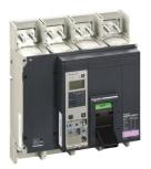
Circuit breaker frame, ComPacT NS1600H, 70kA/415VAC, 1600A, withdrawable, electrically operated, without trip unit, 4P
