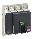
Circuit breaker frame, ComPacT NS800L, 150kA/415VAC, 800A, withdrawable, electrically operated, without trip unit, 4P
