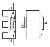
auxiliary wiring plug and socket - for 9 cables - for NS100..250
