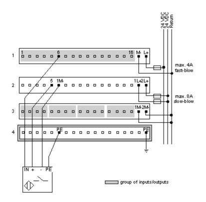
Four-Wire Sensor with a Two-Wire Actuator
