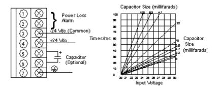
NOTE: A normally closed relay contact rated at 220 Vac, 6A / 30 Vdc, 5A is available on terminals 1 and 2 of the power terminal strip. This contact set may be used to signal input power OFF. The relay will de-energize when input power drops below 8 Vdc.
