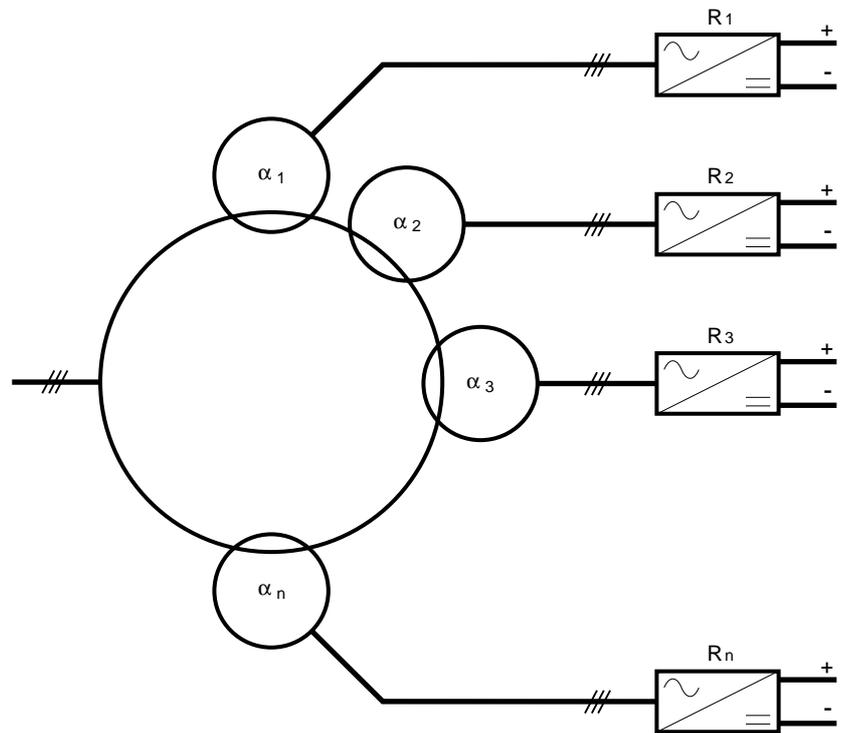
fig. 17: example using  $n$  rectifiers.
