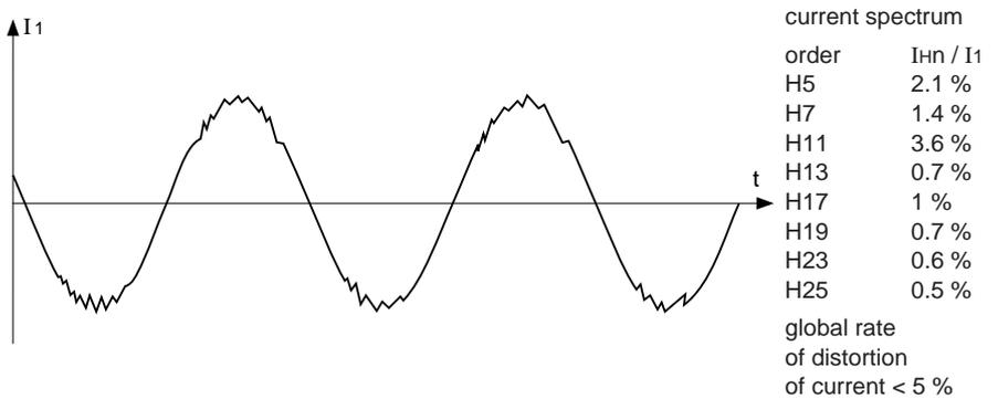
fig. 23: line current of rectifier with harmonic filter.
