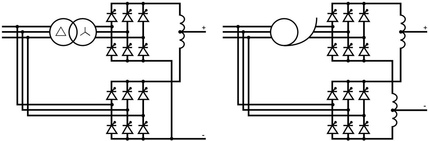
a) circuit connection with power transformer
