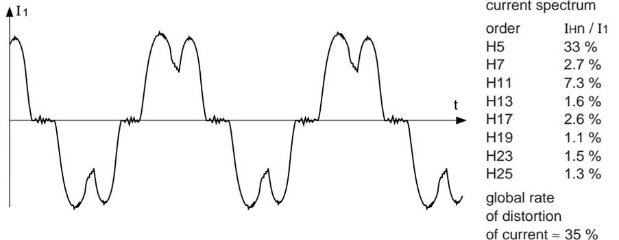
fig. 22: line current of rectifier without harmonic filter.
