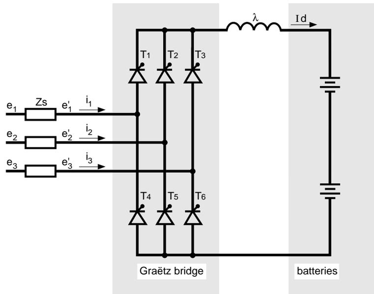
fig. 4: circuit diagram of a Graetz bridge rectifier.
