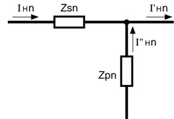
fig. 21: equivalent circuit diagram of filter for harmonics.
