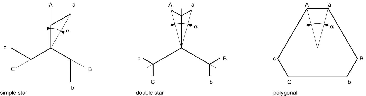
c) various connection circuits for autotransformer
