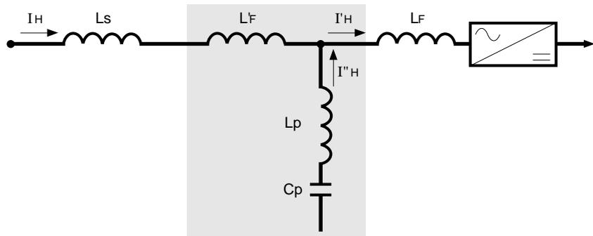
fig. 20: basic circuit of passive filter for harmonics.
