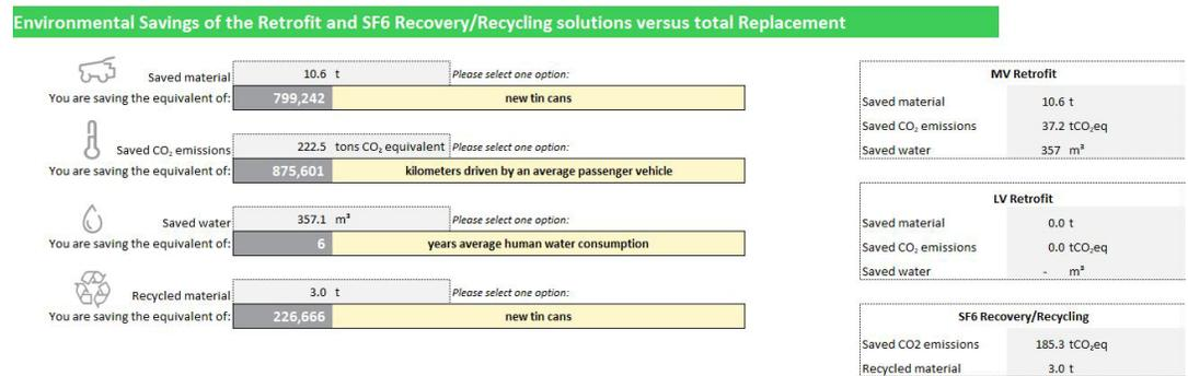
Further environmental benefits can be achieved if the 11 previously described SF<sub>6</sub> technology circuit breakers are recycled. We assume that the obsolete circuit breakers would not have been recycled appropriately, and the SF<sub>6</sub> gas vented to the atmosphere.
