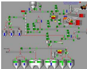
Typical operator HMI screen in the Lafarge application
