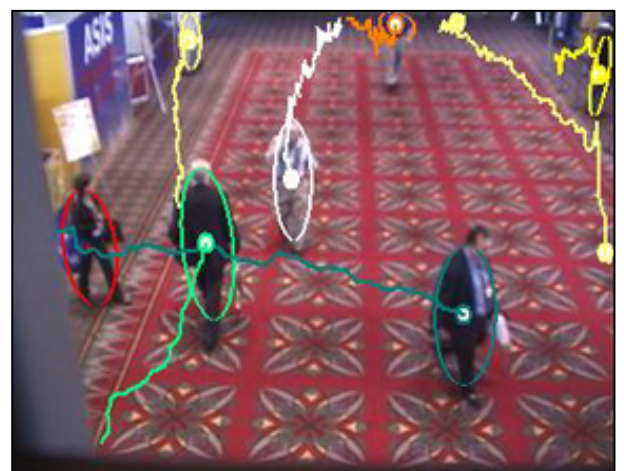
Video analytics software tracks people or objects, and can alarm on types of behavior
